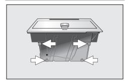
Push the appliance all the way back into the cabinet and center it. If necessary level the unit with the four height adjustable feet. The feet can be turned out up to 3/8" (10 mm).
